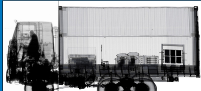
Transmission image of a trailer and cab using CabScan® mode
